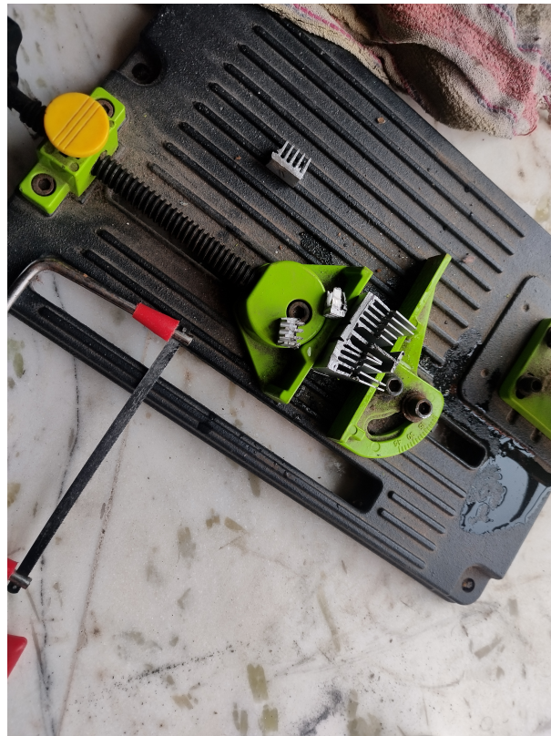
Figure 2: These instruments were used (along with an electric angle cutter) to cut the pieces out of the aluminium heatsink
